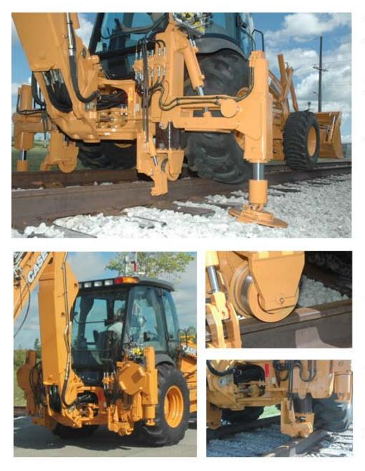
The rear Rail Gear pins where the standard backhoe wing down stabilizers were attached to the backhoe frame.
