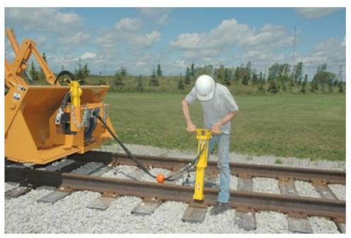
The Attachment used to operate hand held tools is the Tool Circuit with Hose Reel Mount.
